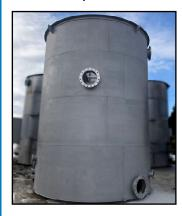
Manufactured of stainless steel or epoxy-coated carbon steel, *Phalanx* utilizes the combined air-water backwash process to clean dual- or mono-media designs to reduce water consumption and optimize cleaning. The addition of an Ortho-Wash™ baffled wash trough guarantees media retention and minimizes filter height.
